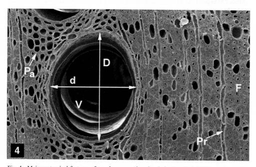
Fig. 4 - Main anatomical features of wood cross section. Symbols: V = Vessel; D = maximum diameter (radial); d = minimum diameter (tangential); Pr = radial parenchyma; Pa = axial parenchyma; F = fibres.
